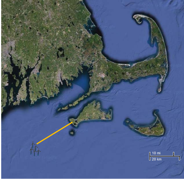
Figure 26a Radial Configuration for Single Wind Farm
